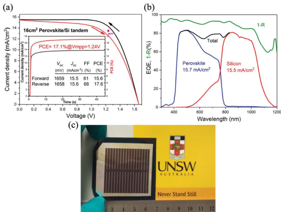
**Fig. 8** (a)  $J$ - $V$  curve and the steady-state PCE in the inset for the champion tandem device on 16 cm<sup>2</sup> using the heavier p++ front emitter for the Si bottom cell. (b) EQE for the corresponding tandem device (black), for the perovskite top cell (blue), and the silicon bottom cell (red). The total absorbance (1-reflectance) of the tandem device is shown by the green line. (c) A photo of a fabricated 16 cm<sup>2</sup> tandem.
