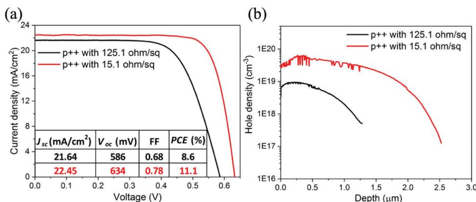
Fig. 4 (a) Current density-voltage ( $J$ - $V$ ) curves of  $\text{Si}$  bottom cells that have different  $\text{p}++$  emitter profiles (black for  $125.1 \text{ ohm sq}^{-1}$  and red for  $15.1 \text{ ohm sq}^{-1}$ ). (b) Doping profiles of the same cells measured with electrochemical capacitance-voltage measurements.
