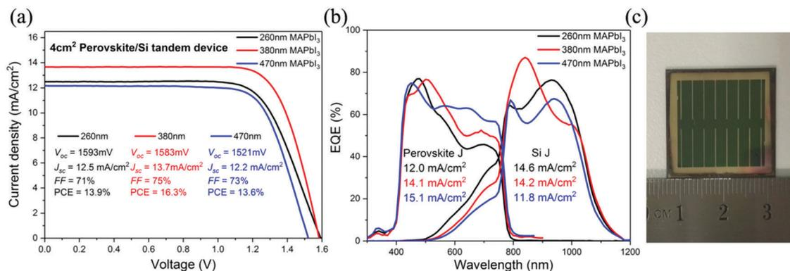
Fig. 2 (a)  $J$ - $V$  curves and (b) EQE of the tandem devices with different thicknesses of the MAPbI<sub>3</sub> perovskite layer (260, 380 and 470 nm). (c) A photo of a fabricated 4 cm<sup>2</sup> tandem device.
