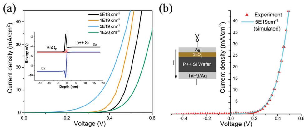
Fig. 3 (a) Simulated dark  $J$ - $V$  curves for the  $\text{SnO}_2/\text{p}++$  silicon interface when the  $\text{p}++$  doping concentration is varied. Inset: Corresponding band diagram taking into account the effect of native  $\text{SiO}_2$ . (b) Dark  $J$ - $V$  characteristics of the  $\text{Ag}/\text{SnO}_2/\text{p}++ \text{Si}/\text{Ag}$  test device (the inset shows the structure of the test device).
