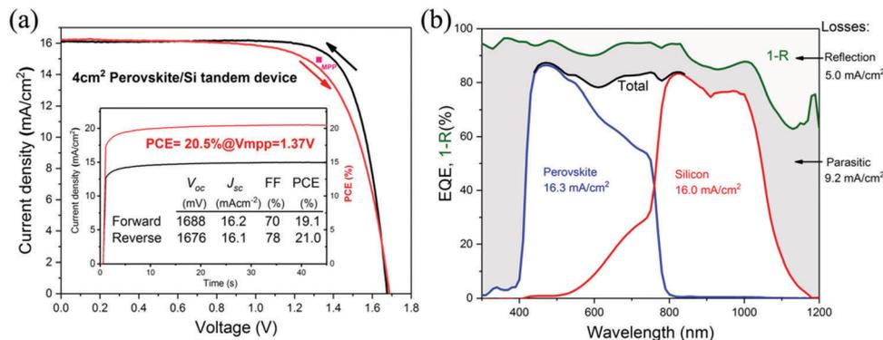
Fig. 7 (a)  $J$ - $V$  curve and in the inset: steady-state PCE of the champion tandem device on 4 cm<sup>2</sup> using the heavier p++ front emitter for the Si bottom cell and with antireflection foil on the front of the tandem. (b) EQE for the corresponding device (black), for the perovskite top cell (blue), and for the silicon bottom cell (red). The total absorbance (1-reflectance) of the tandem device is shown by the green line.
