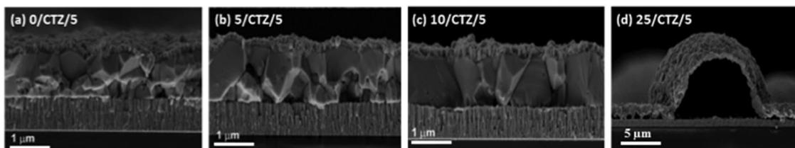
Fig. 6 Cross-sectional SEM micrographs of the completed CZTSe solar cells with different amounts of Ge deposited below the metallic Cu/Sn/Cu/Zn precursor stack: (a) 0 nm Ge below, (b) 5 nm Ge below, (c) 10 nm Ge below, (d) 25 nm Ge below. All precursors had deposited a 5 nm Ge layer on top.
