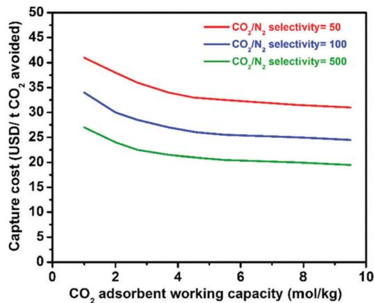
Fig. 2 Relationship between the CO<sub>2</sub> capture cost and CO<sub>2</sub> selectivity/working capacity of solid adsorbents.<sup>9</sup> Figure reproduced with permission from Elsevier.
