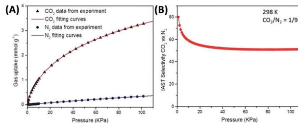
Fig. 7 (A) Single CO<sub>2</sub> and N<sub>2</sub> adsorption isotherms of a microporous carbon material fitted with a dual-site Langmuir–Freundlich model and (B) calculated IAST selectivity for a range of total pressures (0–110 kPa) at a molar CO<sub>2</sub>/N<sub>2</sub> ratio of 1/9.<sup>9</sup> Figure reproduced with permission from the Royal Society of Chemistry.
