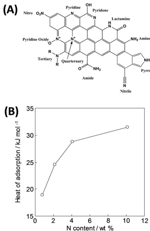
Fig. 9 (A) Various nitrogen species in N-doped carbons<sup>9</sup> and (B) change in the isosteric enthalpy of CO<sub>2</sub> adsorption with nitrogen content for nitrogen-doped polypyrrole-based porous carbons at a surface coverage of ~0.6 mmol g<sup>-1</sup>.<sup>92</sup> (A) Reproduced with permission from the Royal Society of Chemistry. (B) Reproduced with permission from Wiley.
