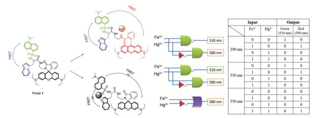
Proposed binding mechanisms of the probe with Fe<sup>3+</sup> and Hg<sup>2+</sup> and the truth table
