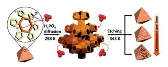
Scheme 1 Illustration of the etching process for MIL-100(Fe). Left: MIL-100(Fe) crystal with hexagonal and pentagonal windows; middle: acid diffusion into tetrahedral channels through hexagonal windows; right: resulting mesopores after etching.
