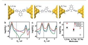
Fig. 4 (a) Relaxed structures of the molecules from DFT. (b) Calculated conductance {A} of the initial state and (c) the protonated state for the molecules shown in Scheme 1c: 1,3Az (red), 4,7Az (blue), and 5,7Az (green). (d) Comparison between the calculated conductance and the experimentally determined conductance. The transmission curves leading to these conductances are shown in Fig. S3-1 of the ESI.†
