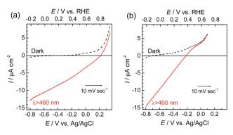
Fig. 1 Current-potential curves of RuRe/CuGaO<sub>2</sub> (a) and RuRe/NiO<sup>31</sup> (b) electrodes under continuous visible-light irradiation ( $\lambda_{ex} > 460$  nm) and under dark conditions. A 50 mM aqueous solution of NaHCO<sub>3</sub> (pH 6.6) saturated with CO<sub>2</sub> was used as the electrolyte.
