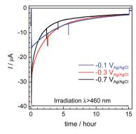
Fig. 6 Time courses of the photocurrent using the RuRe/CuGaO<sub>2</sub> photocathode at various potentials (corresponding to entries 1–3 in Table 1) under irradiation at  $\lambda_{\rm ex}$  > 460 nm.
