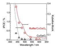
Fig. 2 Dependence on wavelength of the incident-photon-tocurrent efficiencies of the RuRe/CuGaO<sub>2</sub> (red circles) and bare  $CuGaO_2$  (black triangles) electrodes at -0.3 V vs. Ag/AgCl. An aqueous solution containing 50 mM NaHCO<sub>3</sub> saturated with CO<sub>2</sub> was used as the electrolyte (pH 6.6). The diffuse reflectance spectra of these electrodes are also shown: RuRe/CuGaO<sub>2</sub> (red solid line) and CuGaO<sub>2</sub> (black broken line)
