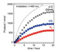
Fig. 4 Time courses of the chemical products (CO and H<sub>2</sub>) and a half amount of electrons passing through the RuRe/CuGaO2 photocathode under continuous visible-light irradiation ( $\lambda_{ex} > 460$  nm) at -0.3 V vs. Ag/AgCl. A 50 mM aqueous solution of NaHCO<sub>3</sub> (pH 6.6) that was saturated with CO2 was used as the electrolyte.
