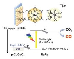
Fig. 3 Reaction scheme of the reduction of CO<sub>2</sub> by the RuRe/CuGaO<sub>2</sub> hybrid photocathode.
