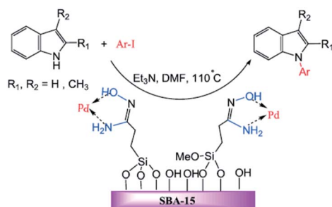
Fig. 25 Palladium-catalysed N -arylation of indoles. Reprinted from ref. 125 with permission of Wiley.
