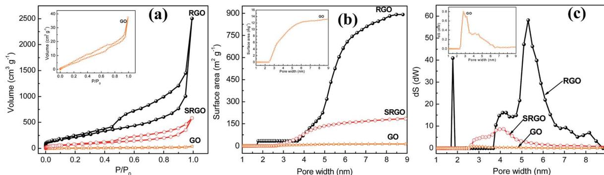
Fig. 4 (a)  $\text{N}_2$  adsorption isotherms of graphene oxide, reduced graphene oxide before (RGO) and after reaction with *in situ*-generated 4-sulphophenyl diazonium cations (SRGO), (b) cumulated surface area vs. pore width of GO, RGO and SRGO, (c) pore size distribution of GO, RGO and SRGO. The insets present the data for GO at a more sensitive scale.
