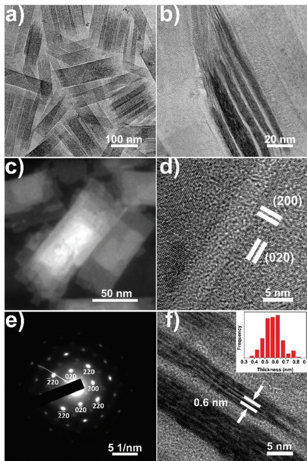
**Fig. 4** Characterization of the as-synthesized ceria ML-nanoplates. (a, b) TEM images; (c) HAADF-STEM image; (e) SAED pattern; (d, f) HRTEM images; the inset in (f) shows the thickness distribution of the layers in the ML nanoplates.
