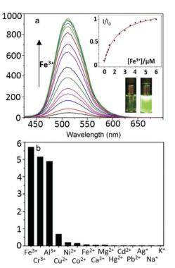
Fig. 2 (a) Steady-state single photon fluorescence spectroscopy ( $\lambda_{\rm ex}$  = 403 nm) of **TNP** (1  $\mu$ M) in ethanol–water (80 : 20, v/v) with a buffer solution of HEPES (10 mM, pH = 7.4) in the presence of different concentrations of aqueous metal ions. Inset: Fluorescence intensity at 515 nm of **TNP** as a function of aqueous Fe<sup>3+</sup> concentration. (b) Fluorescence intensity change of **TNP** (1  $\mu$ M) in the presence of metal ions (10  $\mu$ M).
