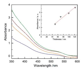
Fig. 4 Plots of the absorbance of the thin films of  $Ta_3N_5$  on quartz with different thicknesses: 50 nm (blue), 70 nm (orange), 99 nm (red), and 122 nm (green). The inset is the absorbance at 350 nm vs. the thickness of the films.
