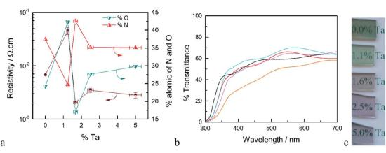
Fig. 1 (a) Resistivity (brown) and atomic% of O (blue) and N (red) of Ta-doped TiO<sub>2</sub> as a function of % Ta. (b) Optical transmittance of Ta-doped TiO<sub>2</sub> films, un-doped TiO<sub>2</sub> (orange), 5.0% Ta (black), 2.5% Ta (red), 1.67% Ta (cyan) and 1.25% Ta (pink). (c) Photographs of the TTO films after annealing in ammonia at 750 °C for 30 min.
