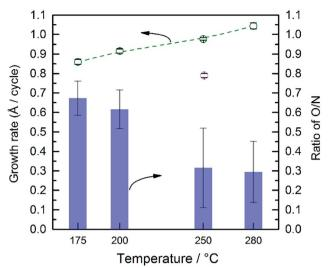
Fig. 2 Growth rate of  ${\rm TaO}_x{\rm N}_y$  (green) and  ${\rm TaO}_x$  (pink) as a function of deposition temperature. Also shown are the ratios of atomic concentrations of O/N (purple) as a function of the deposition temperature found from the EDS analysis.
