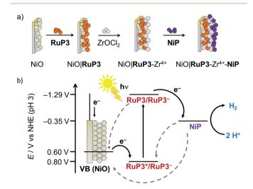
Fig. 2 (a) Supramolecular dye–catalyst assembly on photocathode: layer-by-layer deposition of RuP3, Zr<sup>4+</sup> and NiP on p-type NiO photocathode (see text for details). (b) Energy diagram of the NiO photocathode assembly showing the proposed electron transfer mechanisms (reductive quenching) as black solid arrows and possible recombination pathways as grey dashed arrows between p-NiO, RuP3 and NiP.
