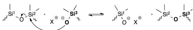
Fig. 7 Siloxane silanol exchange reaction through addition and elimination of a silanolate anion.
