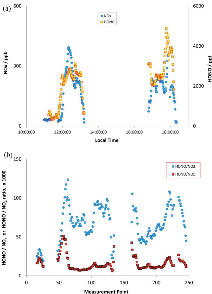
Fig. 8 Measured HONO and  $\text{NO}_x$  (panel a, upper) and HONO/ $\text{NO}_2$  and HONO/ $\text{NO}_x$  ratios (panel b, lower) during on-road measurements, transect from Birmingham to Leicester & return.
