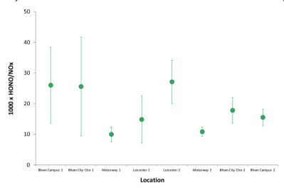
Fig. 11 Mean ( $\pm 1$  standard deviation) HONO/NO<sub>x</sub> ratios observed for each environment, spatially defined, during the on-road transect measurements.
