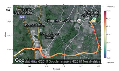
Fig. 10 Enlargement of Fig. 9 – measured HONO (panel a, upper) and  $HONO/NO_2$  ratio (panel b, lower) around the Leicester end of the journey, including open highway, congested major urban artery and urban background sections, from bottom-left to top-right respectively.
