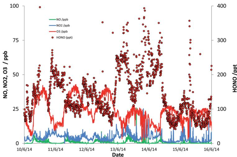
Fig. 1 (Subset of) measured NO, NO<sub>2</sub>, O<sub>3</sub> and HONO data at the University of York campus.
