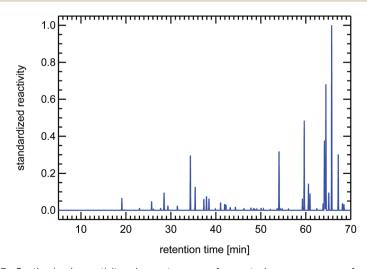
Fig. 17 Synthesized reactivity chromatogram of a petrol passenger car for warm conditions.
