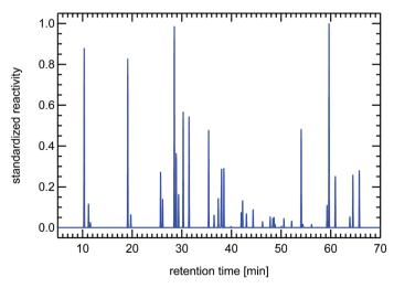
Fig. 21 Synthesized reactivity chromatogram of an air sample taken in 1997 in Munich, "Garmischer Straße".
