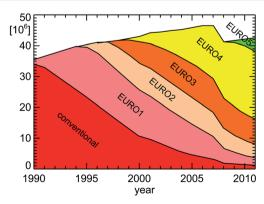
Fig. 8 Vehicle emission regulation categories for passenger cars in Germany for the years 1990–2011; replotted from TREMOD version 5.3 (see ref. 15 and Table 1).
