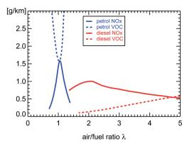
Fig. 3  $NO_x$  and VOC emissions of diesel and petrol passenger cars without catalytic converters; replotted using published mixing ratio measurements (see ref. 6) multiplied with  $\lambda$  to be proportional to g km<sup>-1</sup> and then scaled to the values of Table 1 at  $\lambda=1$  for petrol and  $\lambda=3$  for diesel passenger cars.
