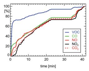
Fig. 5 Normalized cumulative emissions of CO (100% = 2.09 g corresponding to 0.116 g km $^{-1}$ ), CO $_2$  (180 g km $^{-1}$ ), NO (0.149 g km $^{-1}$  as NO $_2$ ), NO $_2$  (0.173 g km $^{-1}$ ), and VOC (0.008 g km $^{-1}$  as HC) derived during measurements of a diesel car (see ref. 7) during a drive of 18.0 km length 27.11.2002 executing a FTP-75-cycle (passenger diesel car, year of manufacture: 2002, 105 kW, DOC, exhaust norm EURO3).
