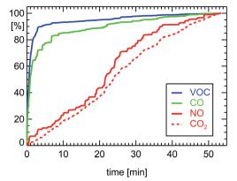
Fig. 4 Normalized cumulative emissions of CO (100% = 23.8 g corresponding to 0.80 g km<sup>-1</sup>), CO<sub>2</sub> (262 g km<sup>-1</sup>), NO (0.205 g km<sup>-1</sup> as NO<sub>2</sub>), and VOC (0.088 g km<sup>-1</sup> as HC) derived during on-board measurements of a petrol car (see ref. 7) during a drive of 29.7 km length 11.07.2001 in Munich (passenger petrol car, year of manufacture: 2000, 85 kW, G-Kat. exhaust norm D4).
