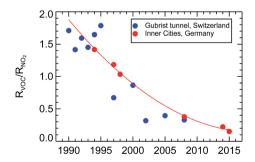
Fig. 25 Observed reactivity ratios of VOC and  $NO_2$ ,  $R_{VOC}/R_{NO_2}$ , over the years 1990–2015 from inner city districts in Germany (this paper) and (scaled, see text) inside the Gubrist road tunnel<sup>40</sup> in Switzerland.
