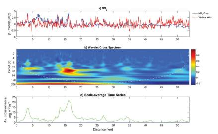
Fig. 2 (a) Variation of  $NO_2$  mixing ratio from the mean and variance of vertical wind speed from the mean, (b) time resolved wavelet cross spectrum, (c) the average cross-covariance between NO<sub>2</sub> mixing ratio and vertical wind, for a typical NE to SW run across London.
