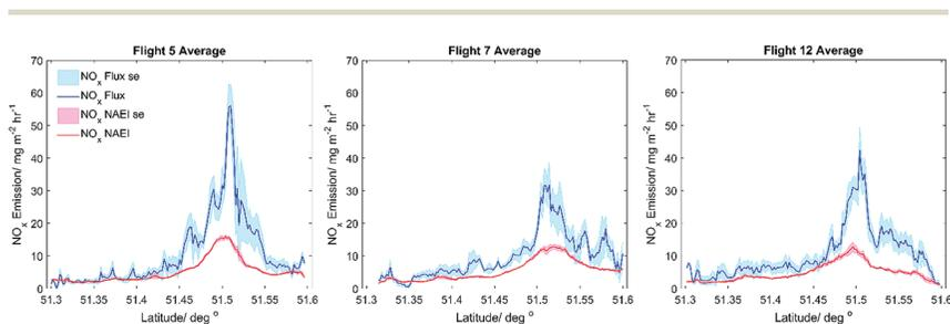
Fig. 5 Average for Flights 5, 7 and 12, measured NO<sub>x</sub> flux plotted in blue with standard error as the shaded blue area. Calculated and scaled NAEI estimates of NO<sub>x</sub> emission are plotted in red, with standard error as the shaded red area.
