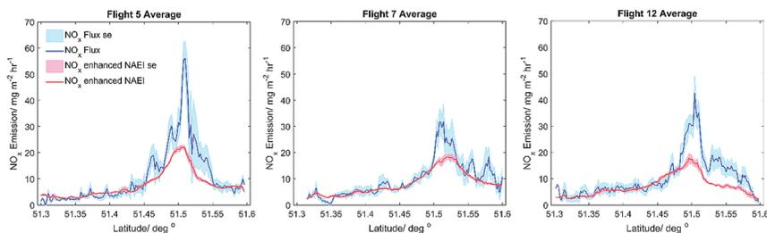
Fig. 7 Average for Flights 5, 7 and 12, measured  $\text{NO}_x$  flux plotted in blue with standard error as the shaded blue area. Calculated and scaled enhanced NAEI estimates of  $\text{NO}_x$  emission are plotted in red, with standard error as the shaded red area.
