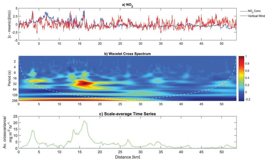
Fig. 2 (a) Variation of NO<sub>2</sub> mixing ratio from the mean and variance of vertical wind speed from the mean, (b) time resolved wavelet cross spectrum, (c) the average cross-covariance between NO<sub>2</sub> mixing ratio and vertical wind, for a typical NE to SW run across London.
