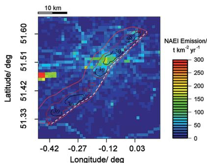
Fig. 3 The contributing footprint area to a typical flight track, dependent on the prevailing wind direction and altitude of flight. The footprint is overlaid onto the NAEI at 1 km<sup>2</sup> grid resolution, coloured to annual NO<sub>x</sub> tonnage emission estimates.
