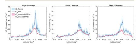
Fig. 7 Average for Flights 5, 7 and 12, measured  $NO_x$  flux plotted in blue with standard error as the shaded blue area. Calculated and scaled enhanced NAEI estimates of  $NO_x$  emission are plotted in red, with standard error as the shaded red area.
