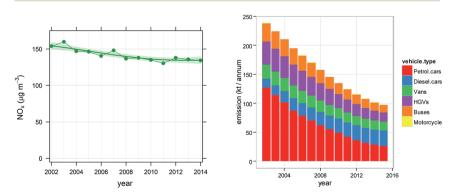
Fig. 1 (a) Trends in the mean concentration of  $NO_x$  across 35 roadside sites in Greater London with at least 10 years of data capture, (b) projected change in urban road transport emissions split by main vehicle type from the NAEI using 2002 as a base year.
