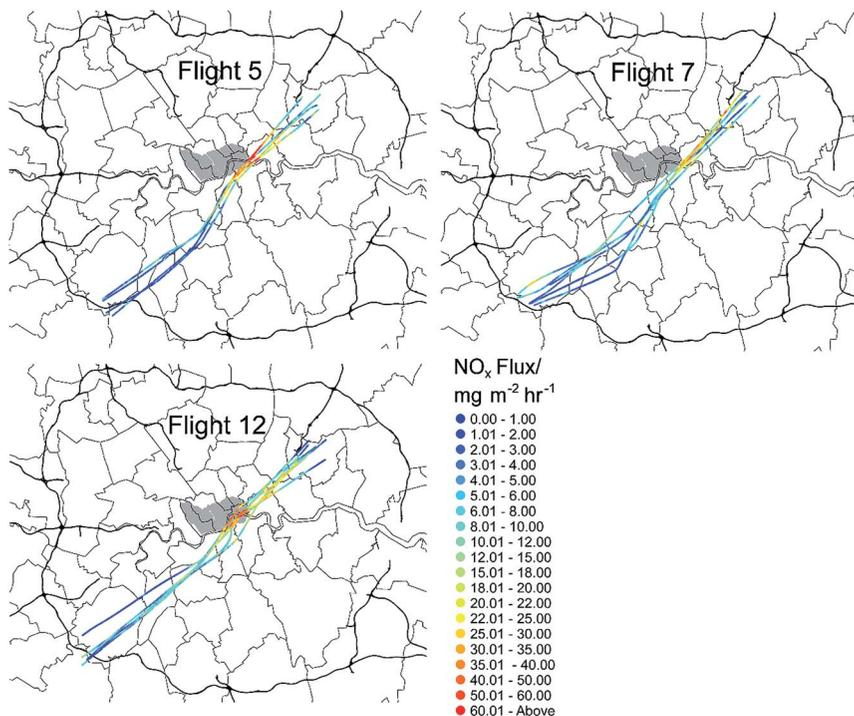
Fig. 4 Tracks of all the flight legs for flights 5 (3rd July 2013 morning), 7 (4th July 2013 afternoon) and 12 (9th July 2013 afternoon), mapped over Greater London, coloured to the measured NO<sub>x</sub> flux. The grey area represents London's Low Emission's Zone (LEZ).
