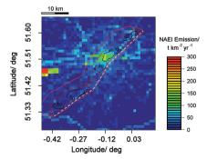
Fig. 3 The contributing footprint area to a typical flight track, dependent on the prevailing wind direction and altitude of flight. The footprint is overlaid onto the NAEI at  $1 \text{ km}^2$  grid resolution, coloured to annual  $NO_x$  tonnage emission estimates.
