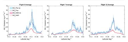
Fig. 5 Average for Flights 5, 7 and 12, measured  $NO_x$  flux plotted in blue with standard error as the shaded blue area. Calculated and scaled NAEI estimates of  $NO_x$  emission are plotted in red, with standard error as the shaded red area.
