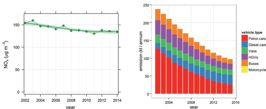
Fig. 1 (a) Trends in the mean concentration of NO<sub>x</sub> across 35 roadside sites in Greater London with at least 10 years of data capture, (b) projected change in urban road transport emissions split by main vehicle type from the NAEI using 2002 as a base year.
