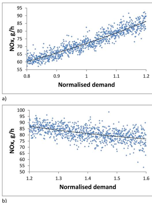
Fig. 2 Total exhaust emissions of NO<sub>x</sub> for a sample section of Gillygate for (a) off-peak and (b) peak demand scenarios.
