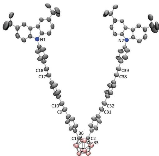
Fig. 1 Crystal structure of **D-3**. Selected bond lengths (Å): C1–C2 1.718(3), C9–C10 1.187(3), C17–C18 1.198(3), C31–C32 1.187(3), C38–C39 1.198(3), C1–N1 19.376, C2–N2 19.376. Hydrogen atoms have been omitted for clarity.
