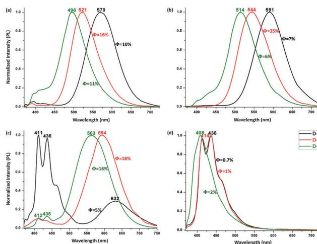
Fig. 3 Normalized PL spectra of **D-1**, **D-2** and **D-3** (2  $\mu\text{M}$ ) in  $\text{C-C}_6\text{H}_{12}$  (a),  $\text{CCl}_4$  (b), toluene (c) and  $\text{CHCl}_3$  (d), with excitation at 350 nm.
