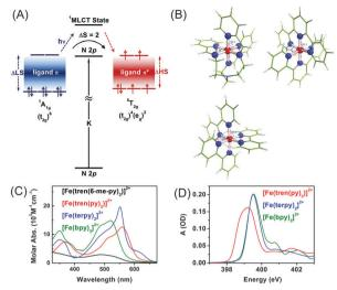
Fig. 4 (A) Schematic of probing a Fe(II) complex in O<sub>h</sub>-symmetry at the N K-edge (1s spectroscopy). (B) Molecular structures of  $[Fe(tren(py)_3)]^{2+}$ ,  $[Fe(terpy)_3]^{2+}$ , and  $[Fe(bpy)_3]^{2+}$ . (C) Optical absorption spectra showing MLCT bands of the three Fe complexes. (D) Transmission N K-edge XAS spectra of solid [Fe(tren(py)<sub>3</sub>)]<sup>2+</sup> (red), [Fe(terpy)<sub>3</sub>]<sup>2+</sup> solution (blue), and  $[Fe(bpy)_3]^{2+}$  solution (green).
