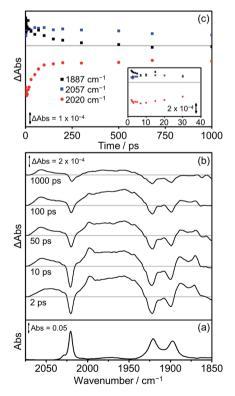
Fig. 11 FTIR and TRIR spectra of Dyad 2 Br in THF: (a) FTIR ground state spectrum; (b) TRIR difference spectra taken between 2, 10, 50, 100 and 1000 ps after flash photolysis at 560 nm; (c) TRIR single point kinetic traces for the CS product (black squares, 1887 cm<sup>-1</sup>), the ground state bands (red dots, 2020 cm<sup>-1</sup>) and the <sup>3</sup>MLCT excited state (blue squares, 2057 cm<sup>-1</sup>). Inset shows expansion of the first 40 ps.
