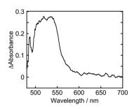
Fig. 7 Time-resolved UV-vis absorption spectrum at 100 ns after the laser excitation: a DMF-TEOA (5:1 v/v) solution containing Ru (0.3 mM) and BI(OH)H (0.1 M) was irradiated at  $\lambda_{\rm ex}=532$  nm with a Nd:YAG pulse laser under degassed conditions at room temperature.
