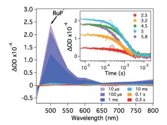
Fig. 2 Transient absorption spectra of RuP (4  $\mu$ M) in the presence of AA (0.1 M) at pH 4.5 as a function of time delay. The inset shows the corresponding kinetics probed at  $\lambda=500$  nm in the pH range between 2.5 and 5.8. The samples were excited at  $\lambda=355$  nm.
