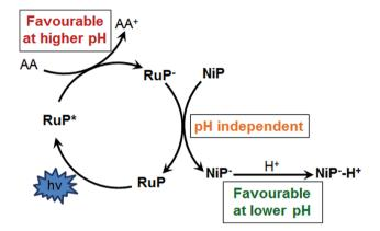
Scheme 1 Schematic representation of the reductive electron transfer mechanism between RuP and NiP in the presence of ascorbic acid as sacrificial electron donor.
