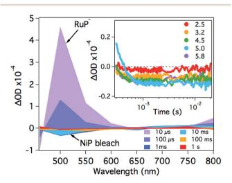
Fig. 3 Transient absorption spectra of a RuP (4  $\mu$ M) and NiP (8  $\mu$ M) mixture in the presence of AA (0.1 M) at pH 4.5 as a function of time delay. The inset shows the time profile of the negative signal monitored at  $\lambda=500$  nm, assigned to the loss of ground state absorption of NiP in the pH range studied. The samples were excited at  $\lambda=355$  nm.
