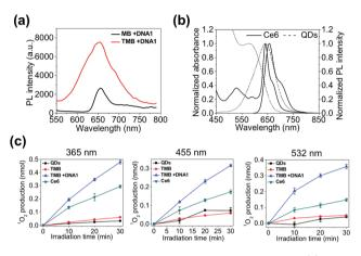
Fig. 3 In vitro evaluation of theranostic efficacy of TMB. (a) Photoluminescence spectra of DNA1-activated TMB and MB (same Ce6 concentration) excited at 405 nm. (b) Normalized absorption spectra and photoluminescence spectra of CdTe/CdS/ZnS QDs and Ce6 molecules. (c) Quantification of  $^{1}O_{2}$  generation by QDs, TMB, DNA1-activated TMB, and free Ce6 (same Ce6 concentration) irradiated at 365 nm, 455 nm, and 532 nm for 10, 20, and 30 minutes.
