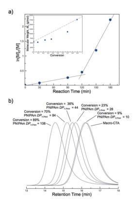
Fig. 5 Data from the PITSA chain extension of a N,N-dimethylacrylamide (DMA) and acrylic acid (AA) containing macro chain transfer agent, [polyDMA34-b-poly(DMA14-co-AA6)], with N-isopropylacrylamide (NIPAm) at 70 °C. (a) First-order kinetics plot showing an increase in rate during the polymerization. Inset:  $M_n$  vs. conversion. (b) SEC traces showing unimodal distributions shifting to higher molecular weights as the polymerization proceeds.
