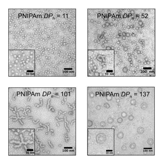
Fig. 4 Transmission electron microscopy of the unpurified crosslinked polymer aggregates showing the progression of nanoparticle morphology as the poly(N-isopropylacrylamide) degree of polymerization (PNIPAm DP<sub>n</sub>) increased (2% uranyl acetate aqueous solution negative stain).
