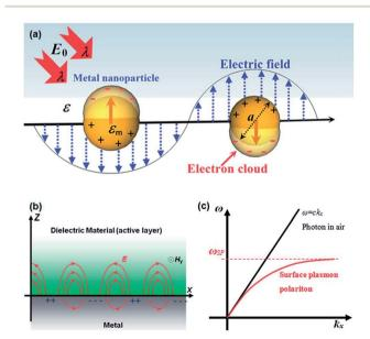
Fig. 1 (a) Schematic representation showing the coherent oscillation of conduction band electrons induced by the interaction of light with light of wavelength  $\lambda$ . (b) Schematic illustration of the surface plasmon polariton modes excited at the metal–dielectric interface. (c) Dispersion curve of surface plasmon polariton (SPP) mode, where a momentum mismatch exists between the light and the SPP. Figure reproduced with permission from ref. 36.
