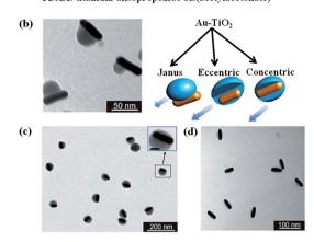
Fig. 6 (a) Preparation scheme and (b–d) TEM images of  $TiO_2$ -coated gold nanorods with (b) Janus, (c) eccentric, and (d) concentric geometries. Figure reprinted with permission from ref. 77.
