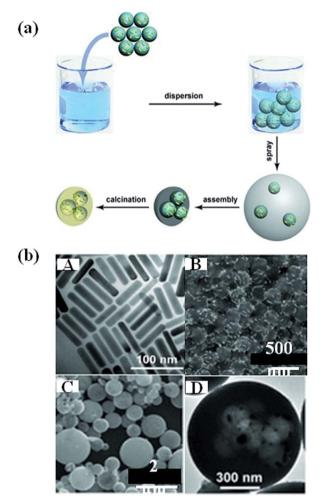
Fig. 8 (a) Schematic representation showing the preparation of the noble metal nanocrystal-embedded hollow mesoporous oxide microspheres through the aerosol-assisted self-assembly process. (b) A: TEM image of Au NR; B: SEM image of polystyrene attached by Au NR; C and D: SEM image of Au nanorods embedded in TiO<sub>2</sub>. Figure reproduced with permission from ref. 89.
