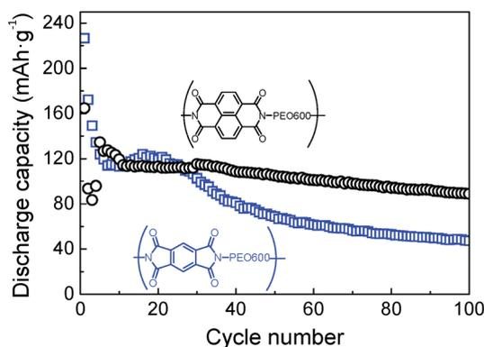
Fig. 8 Discharge capacities versus cycle number for pyromellitic polyimide-*b*-PEO600 (□) and naphthalene polyimide-*b*-PEO600 (○) at 1Li<sup>+</sup>/5 h rate.
