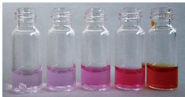
Fig. 10 Color of the leachate when the amount of NdFeB magnet oxide powder, dissolved in 1 mL of diluted HCl and at constants n(\text{HCl})/n(\text{Ln}) ratio of 3.5, was increased from left to right. The purple colour is characteristic for neodymium and the orange colour is due to a small amount of dissolved iron.
