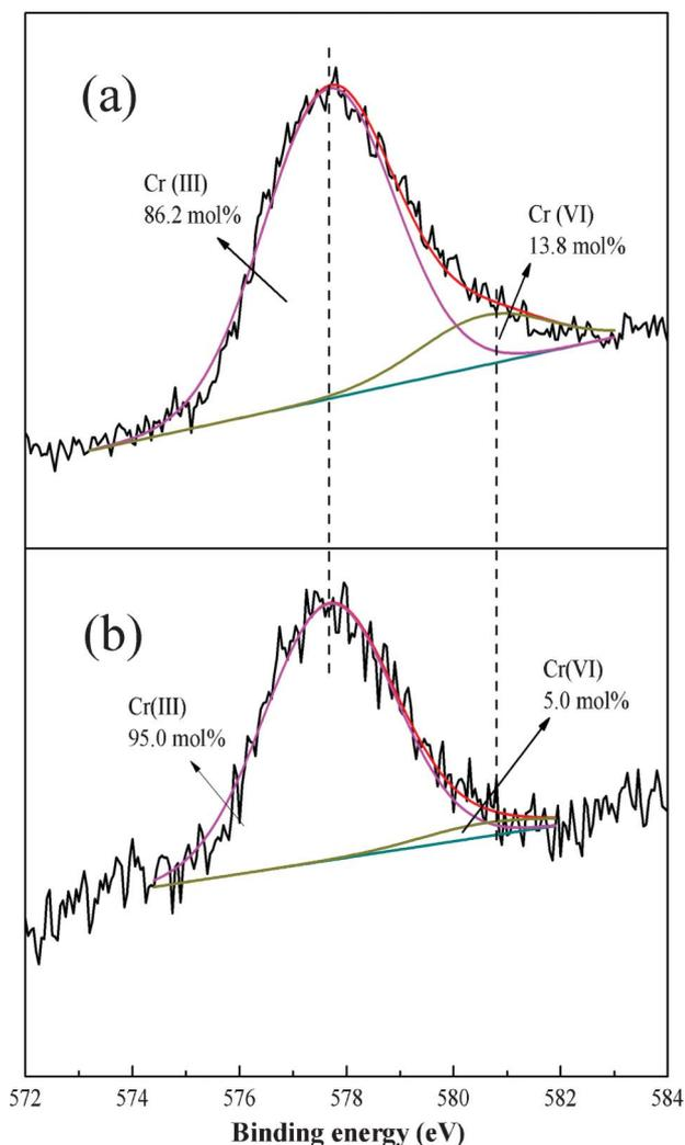
**Fig. 12** Cr 2p<sub>3/2</sub> core level spectra of PAN/PANI nanofiber mat after Cr(vi) adsorption (a), and regeneration (b).
