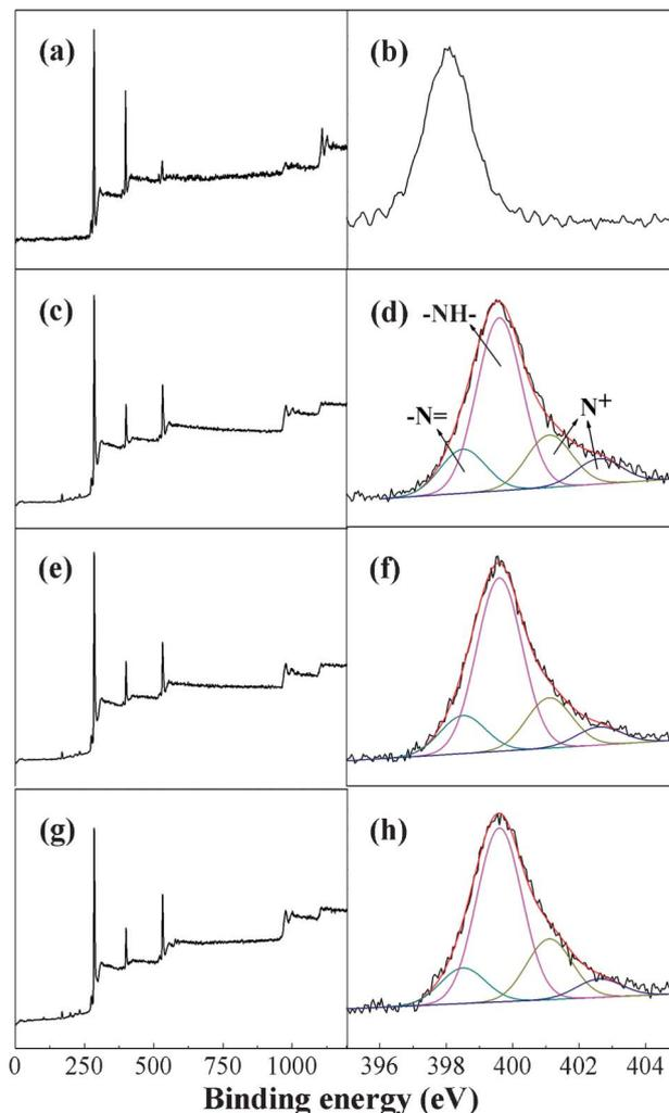
**Fig. 2** XPS wide scan and N 1s core level spectra of pure PAN nanofibers (a and b), and PAN/PANI nanofibers prepared at different polymerization temperatures: 0 °C (c and d), 16 °C (e and f), 35 °C (g and h).
