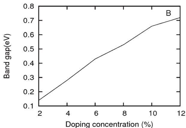
**Fig. 5** Band gap in increasing order of doping concentrations for a boron doped graphene sheet. The isomers with highest band gap are chosen.
