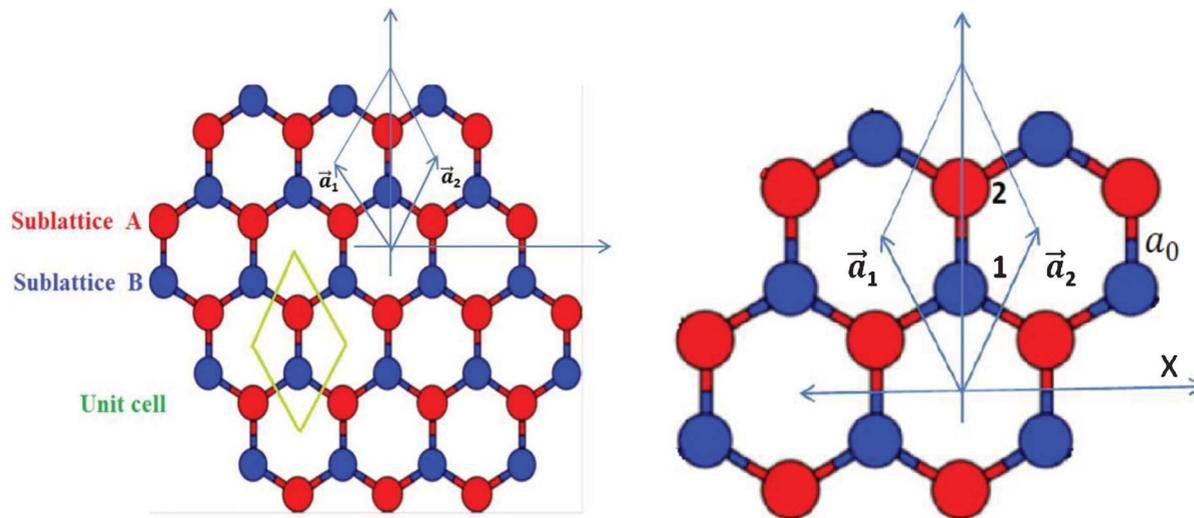
**Fig. 1** A schematic presentation of a graphene sheet. Each Bravais lattice unit cell includes two nonequivalent sites, which are denoted by A and B. A blown-up image of the unit cell is shown separately;  $a_1$  and  $a_2$  are the primitive vectors.
