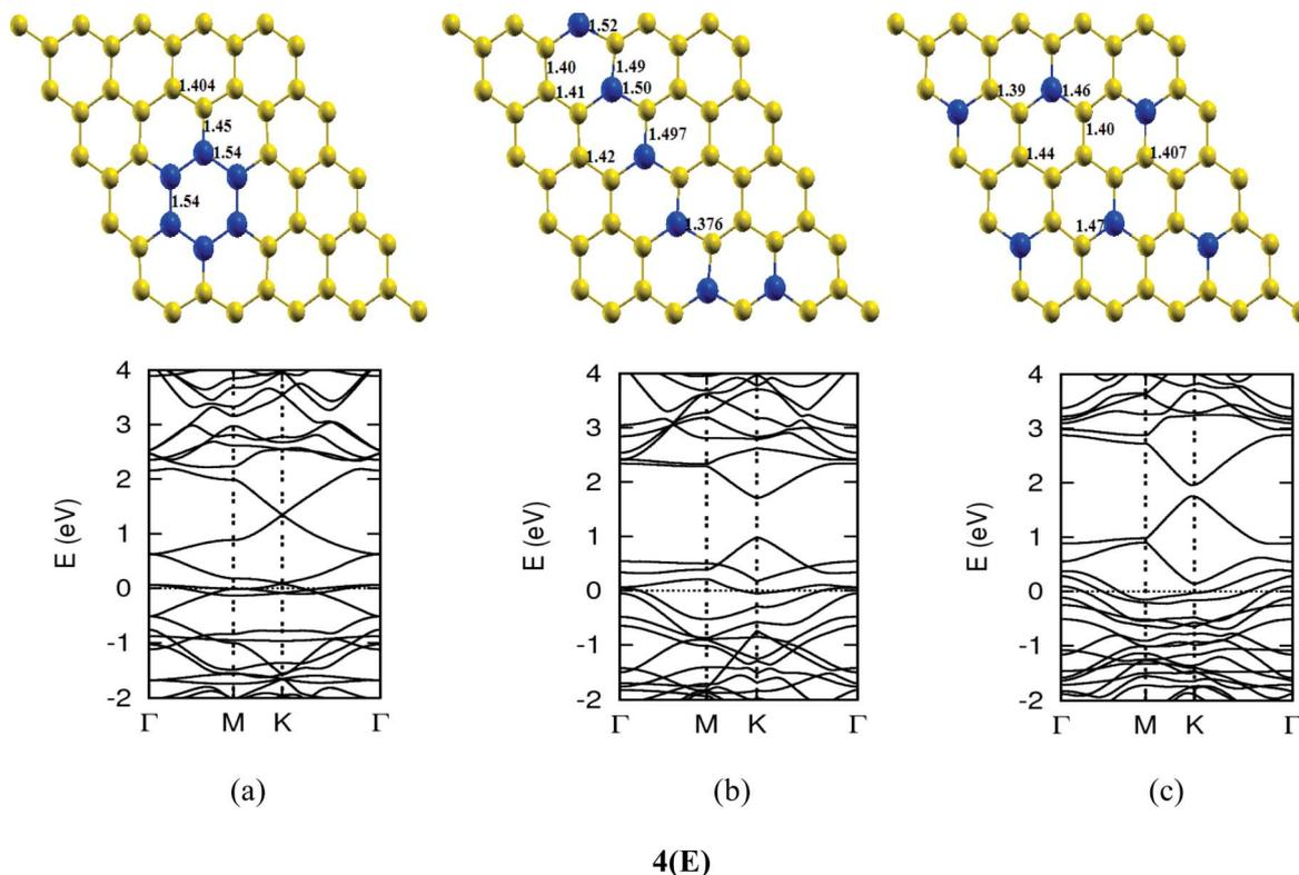
**Fig. 4-3** Some optimized geometries and band structures of two, three, four, five and six B atom doped graphene sheet in (A), (B), (C), (D) and (E), respectively. The upper rows in these show geometrical structures and bottom rows present the band structures.
