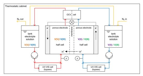
Fig. 2 Experimental setup of the AVRFB test rig used in this work. Red lines indicate the loop of the electrolyte solution in the V(v)/V(v) half-cell, blue lines indicate that of the V(II)/V(III) half-cell, the dashed line represents an electrical conductor, yellow lines indicate the nitrogen loop. For simplicity, the potentiostat, optical fibers, and the UV-Vis spectrometer are not shown
