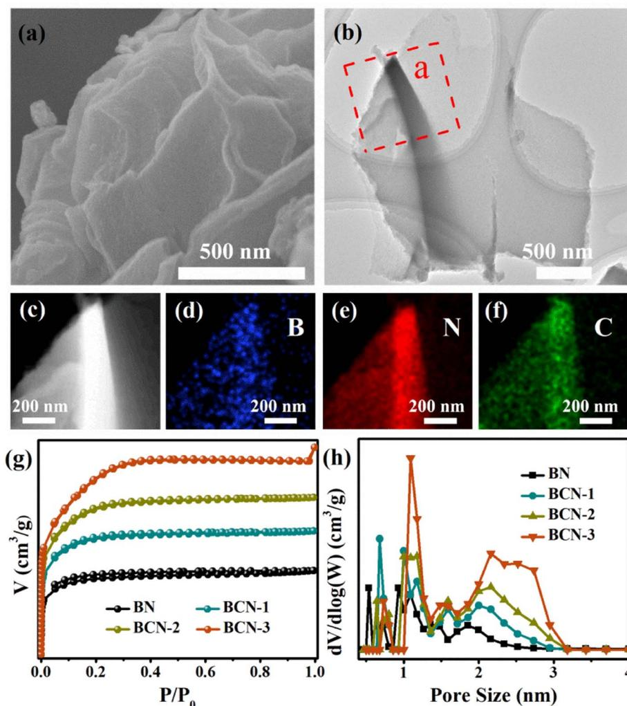
Fig. 3 (a) SEM image of the BCN-2 sample, (b) TEM image of the BCN-2 sample, (c–f) element mapping images of the BCN-2 sample, (g) N<sub>2</sub> adsorption–desorption isotherm plots of all samples and (h) the pore size distribution of all samples.
