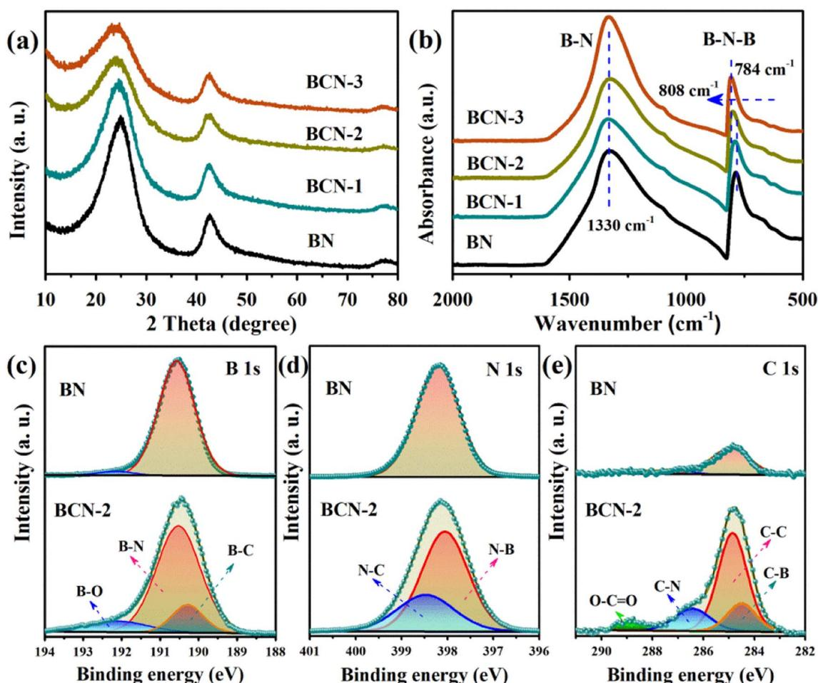
Fig. 2 (a) XRD patterns of all the samples, (b) FT-IR spectra of all the samples, and XPS spectra of (c) B 1s, (d) N 1s and (e) C 1s for the BN and BCN-2.
