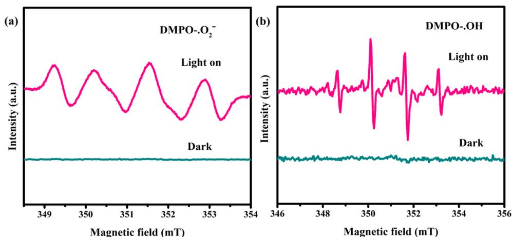
Fig. 8 DMPO EPR spin-trapping of the BCN-2 sample for <sup>•</sup>O<sub>2</sub><sup>-</sup> (a) and <sup>•</sup>OH<sup>-</sup> (b) radicals.
