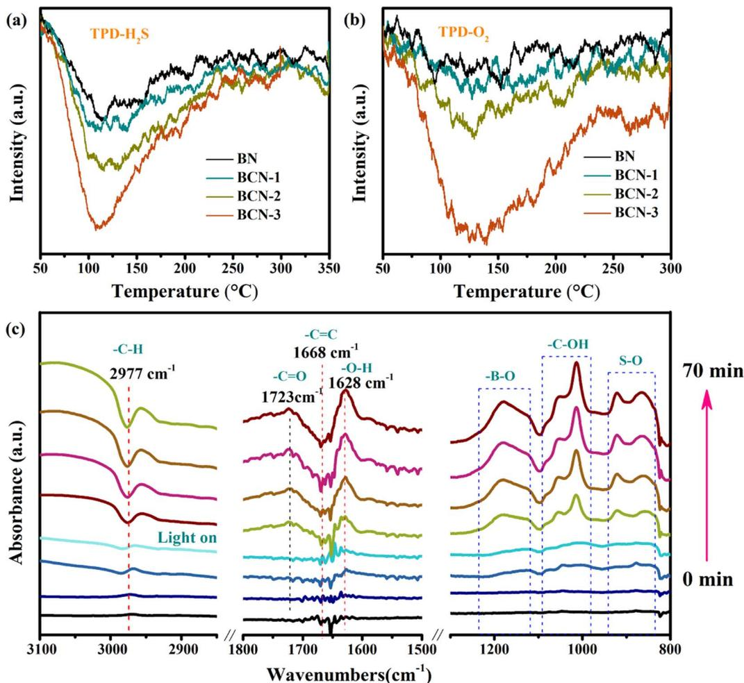
Fig. 7 (a) The temperature-programmed desorption curves of H<sub>2</sub>S for all the samples, (b) the temperature-programmed desorption curves of O<sub>2</sub> for all the samples, (c) DRIFTS test for photocatalytic H<sub>2</sub>S removal over the BCN-2 sample.
