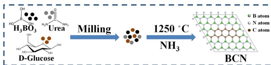
Fig. 1 Schematic diagram of the synthesis of BCN samples.
