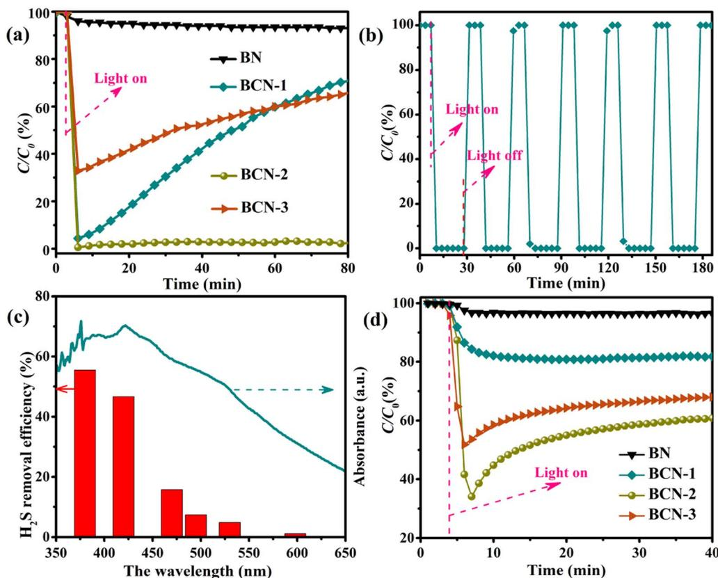
Fig. 6 (a) Photocatalytic H<sub>2</sub>S removal activity of all the samples, (b) photocatalytic activity testing of the BCN-2 sample under light on–off cycles, (c) photocatalytic activity testing of the BCN-2 sample under different monochromatic wavelengths and (d) photocatalytic NO purification of all the samples.
