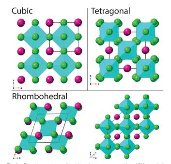
Fig. 1 Crystal structure of cubic aristotype perovskite,  $ABX_3$ , and the tetragonally and rhombohedrally distorted variants. In all three structures the A-site atoms are shown in purple, the X-site atoms are green and the B-site atoms are within the green  $BX_6$  octahedra. The solid black lines outline the crystallographic unit-cell in each structure.
