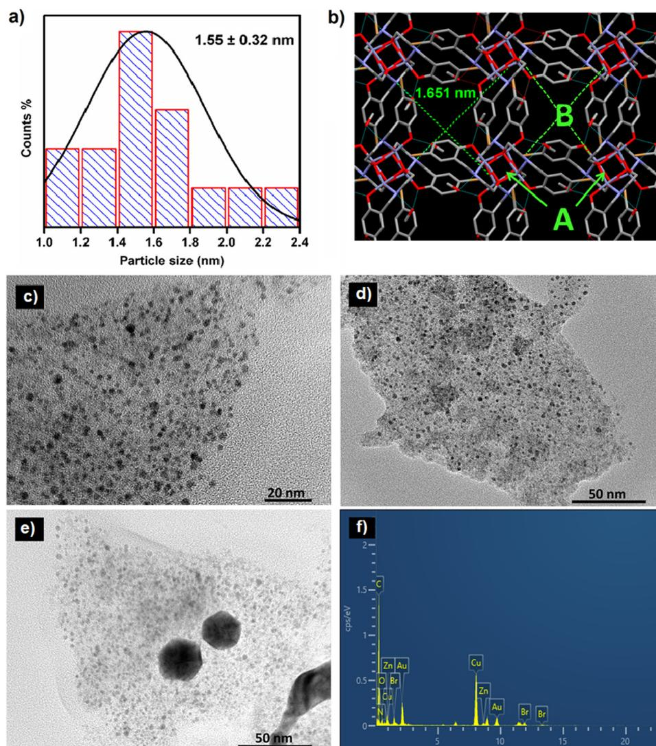
Fig. 4 (a) Particle size distribution of AuNPs, (b) crystal image of the Zn cubane template showing void 'B' of size 1.651 nm, (c)–(e) HR-TEM images of  $\text{ZnCC@AuNPs}$  at different mass loadings, and (f) elemental distribution analysis of  $\text{ZnCC@AuNPs}$ .
