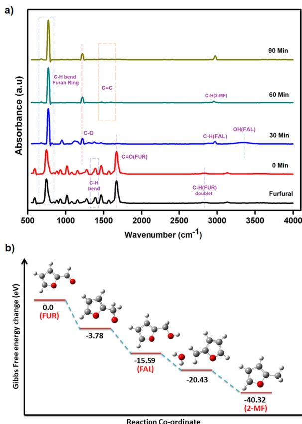
Fig. 8 (a) *In situ* ATR-IR spectra of furfural (FUR) conversion to 2-methylfuran (2-MF) with furfuryl alcohol (FAL) as an intermediate at  $60\text{ }^\circ\text{C}$  for 90 min in *i*-PrOH at regular intervals of 30 min and (b) energy profile diagram of catalytic conversion of furfural (FUR) to 2-methylfuran (2-MF).
