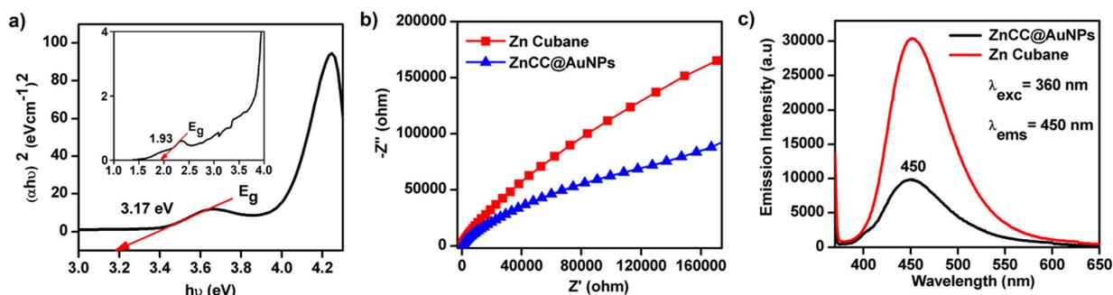
Fig. 6 (a) Tauc plot of ZnCC@AuNPs showing the band gap  $E_g$  (inset: magnified view of the Tauc plot showing a weak band due to LSPR), (b) EIS of Zn cubane and ZnCC@AuNPs, and (c) photoluminescence response of Zn(II) cubane and ZnCC@AuNPs.
