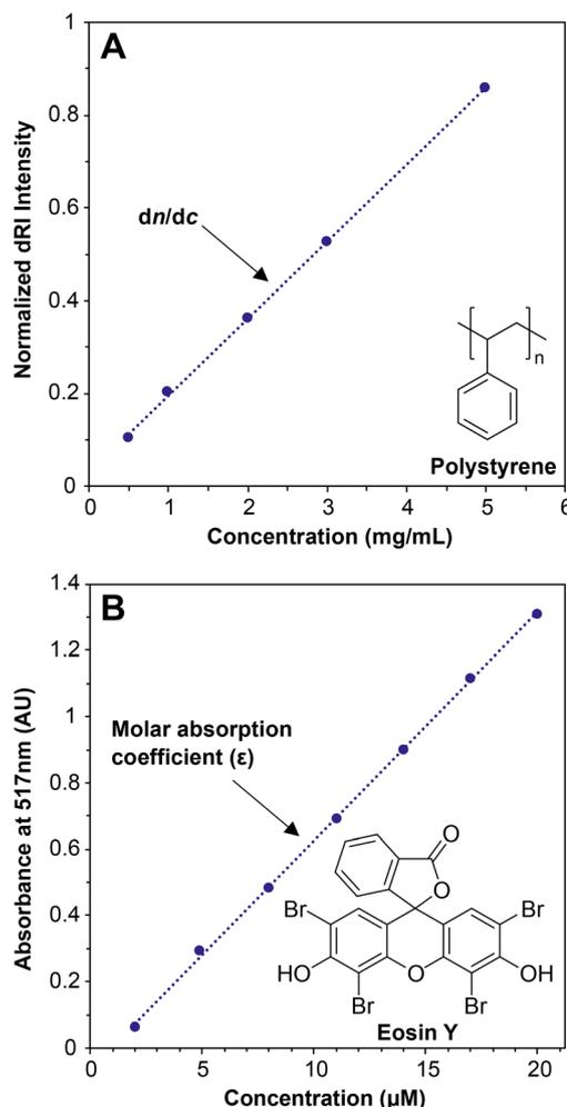
**Fig. 1** (A) Offline  $dn/dc$  experiment using various concentrations of a nominal  $30 \text{ kg mol}^{-1}$  polystyrene (PS) standard in THF, where the slope is equal to the  $dn/dc$ ; (B) UV-vis experiment using various concentrations of eosin Y in water, where the slope is equal to the molar absorption coefficient ( $\epsilon$ ).
