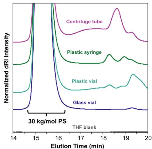
Fig. 5 SEC-MALS chromatograms of a 30 kg mol<sup>-1</sup> PS standard prepared with commonly used plastic laboratory consumable products. All samples were quickly filtered through a 0.22 μm polytetrafluoroethylene (PTFE) syringe filter and added to glass autosampler vials.
