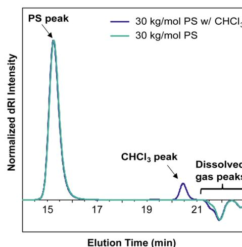
Fig. 6 Overlaid SEC-MALS chromatograms of a 30 kg mol<sup>-1</sup> PS standard in THF (teal trace) and a 30 kg mol<sup>-1</sup> PS standard in THF doped with 1% CHCl<sub>3</sub> as a representative small molecule contaminant (purple trace), which appears at an elution time of 20.5 min. Dissolved gas peaks have a negative inflection and appear at 21–23 min elution time.
