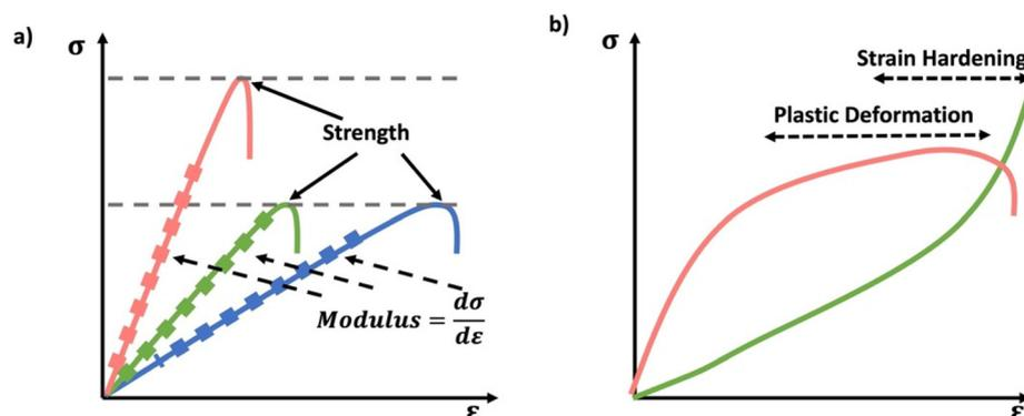
**Scheme 10** (a) Schematic stress-strain curves, showing strength as the peak of the stress-strain curve and modulus as slope of stress-strain curve (b) examples of non-linear stress-strain behavior of plastic deformation and strain hardening/stiffening. Plastic deformation leads to a plateau in stress strain properties typically after a yield point, where linearity in the stress strain curve breaks down. Strain hardening manifests a rapid rise of stress with applied strain.
