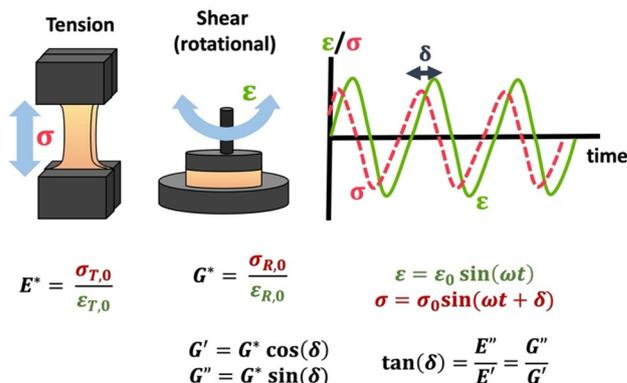
**Scheme 12** Schematic of tensile DMA and SAOR, including  $\sigma$  response to sinusoidally applied  $\epsilon$ , and the complex moduli  $E^*/G^*$  and the storage ( $E'/G'$ ) and loss ( $E''/G''$ ) moduli. Note that  $\sigma_{T,0}$ ,  $\epsilon_{T,0}$ ,  $\sigma_{R,0}$ , and  $\epsilon_{R,0}$  are given in Table 1.
