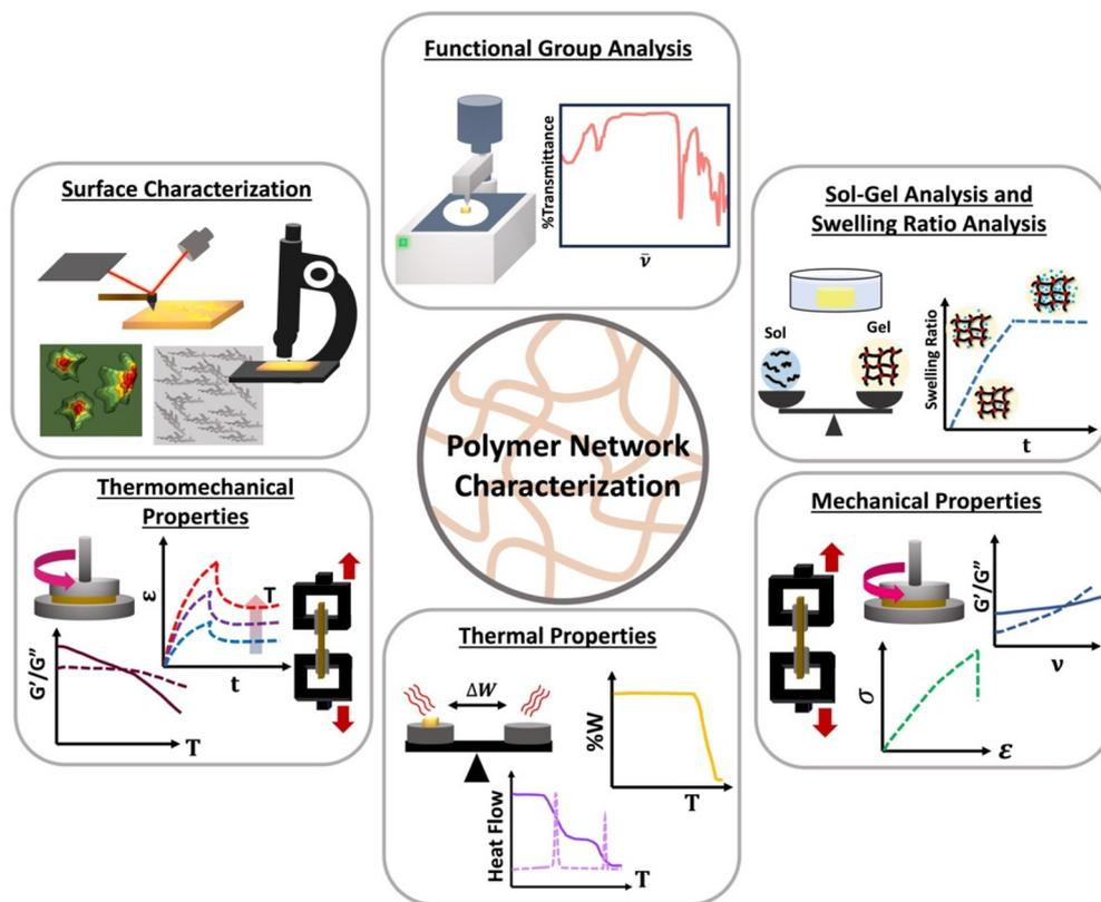
**Scheme 5** Different characterization methods of polymer networks; functional group analysis, sol–gel analysis, swelling ratio analysis, thermal analysis, thermomechanical analysis, and surface characterization.
