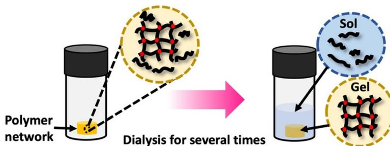
**Scheme 7** Gel extraction process: the crosslinked network is dissolved in an appropriate solvent for a specified duration. Subsequently, the weights of the dried sol fraction and gel fraction are measured. Sol–gel fraction is quantified using eqn (1).
