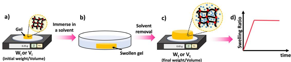
**Scheme 8** Swelling process: (a) take the dry weight/volume of the material, (b) swell the material in an appropriate solvent for a given time ( $t$ ), (c) take the wet weight/volume of the swollen material, (d) calculate the swelling ratio using the eqn (3) and (4) and plot the SRs against the time to study the material's swelling kinetic profile.
