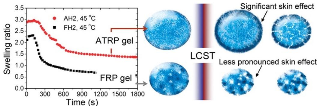
**Fig. 3** (Left) Swelling ratio over time for 2-(2-methoxyethoxy)ethyl methacrylate networks above the LCST for both ATRP and FRP networks. Right shows skin like effects on the periphery of the network (reproduced from ref. 75 with permission from American Chemical Society, copyright 2010).
