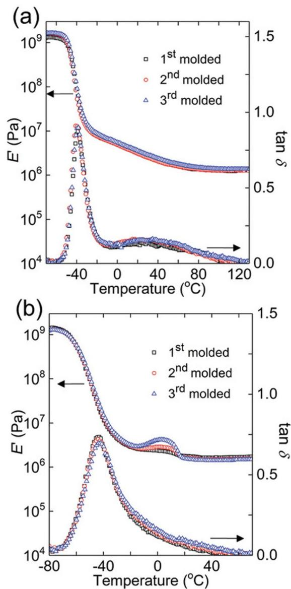
**Fig. 8** Dynamic mechanical responses of (a) PB networks and (b) PTMO networks:  $E'$  and  $\tan \delta$  as functions of temperature for 1st molded (squares), 2nd molded (circles), and 3rd molded (triangles) samples (reproduced from ref. 112 with permission from John Wiley and Sons, copyright 2019).
