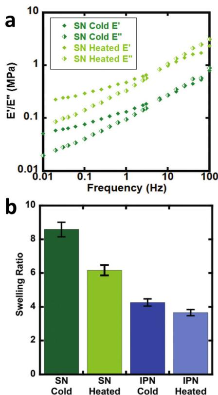
**Fig. 6** (a) Dynamic mechanical analysis showing the increase in modulus upon heating the dynamically crosslinked polymers (b) Reduction of the swelling ratio for the same materials as well as interpenetrated networks (reproduced from ref. 103 with permission from Royal Society of Chemistry, copyright 2021).
