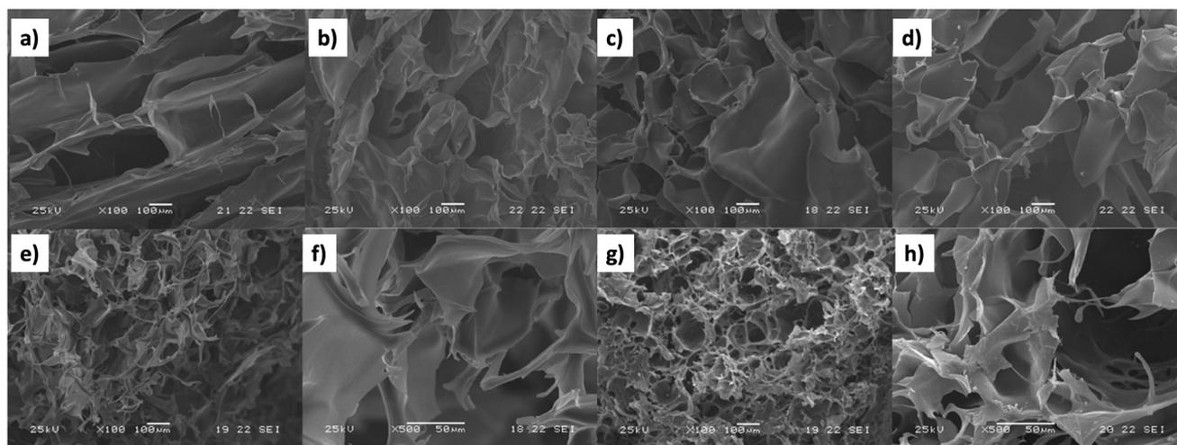
**Fig. 9** SEM images of HEC<sup>90</sup>/AAC hydrogels ( $M_v = 90\,000$ ) containing (a) 5%, (b) 10%, (c) 20%, and (d) 30% AAC, HEC<sup>1300</sup> (e and f) and HEC<sup>1300</sup>/AAC gels ( $M_v = 130\,000$ ) containing 5% AAC (g and h) (magnification:  $\times 100$  a and g;  $\times 500$  f and h) (reproduced from<sup>115</sup> with permission from Elsevier, copyright 2017).
