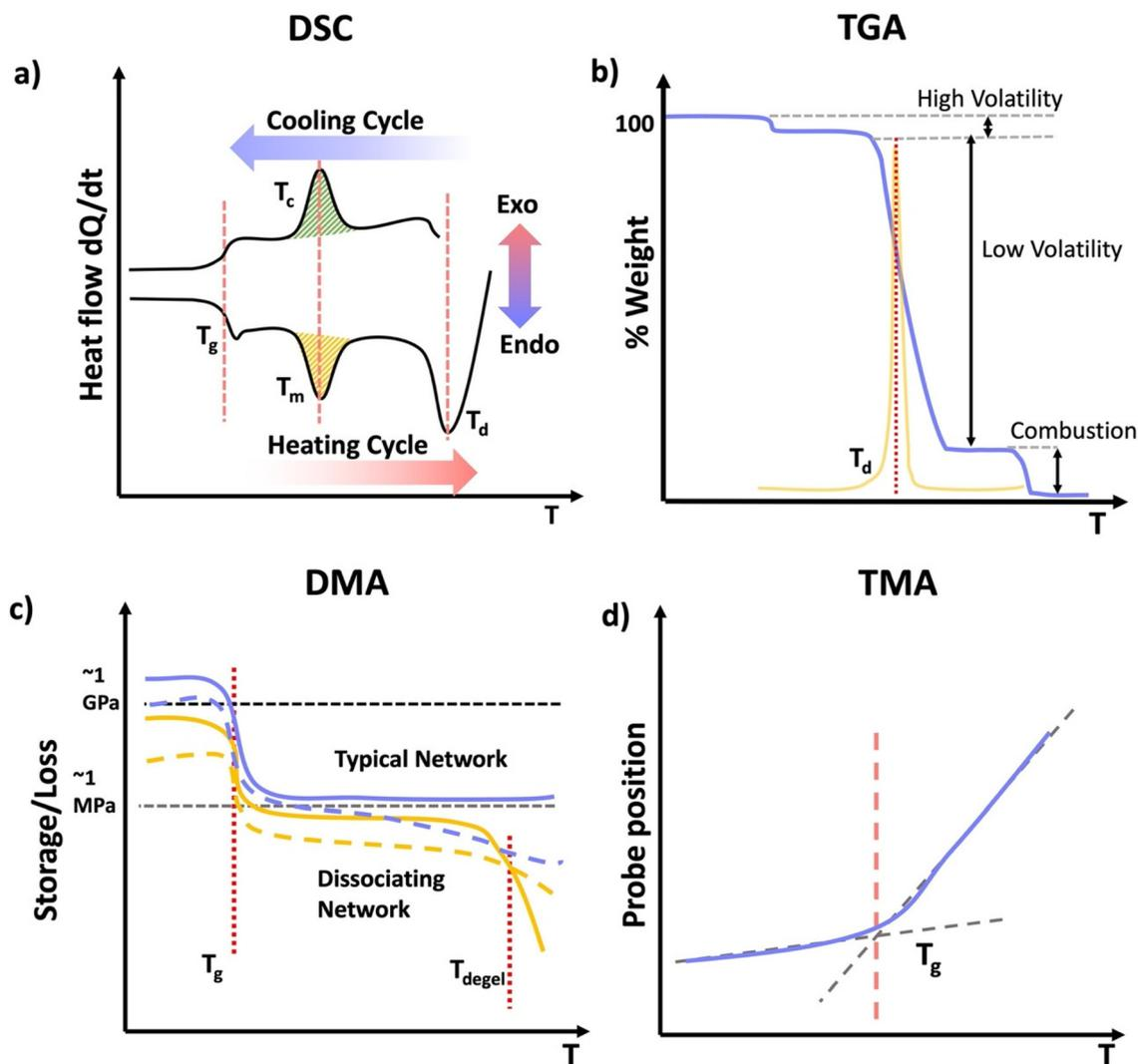
**Scheme 13** (a) Typical DSC curve with the specific regions; glass transition, melting, crystallization, and degradation. (b) Typical TGA curve for a polymeric material showing loss of a volatile compound, and degradation. (c) Typical DMA or SAOR profile for a typical permanently crosslinked network in blue and a dissociating network in orange highlighting  $T_g$  and dissociation of the orange network. (d) Typical TMA position profile used to identify  $T_g$ .
