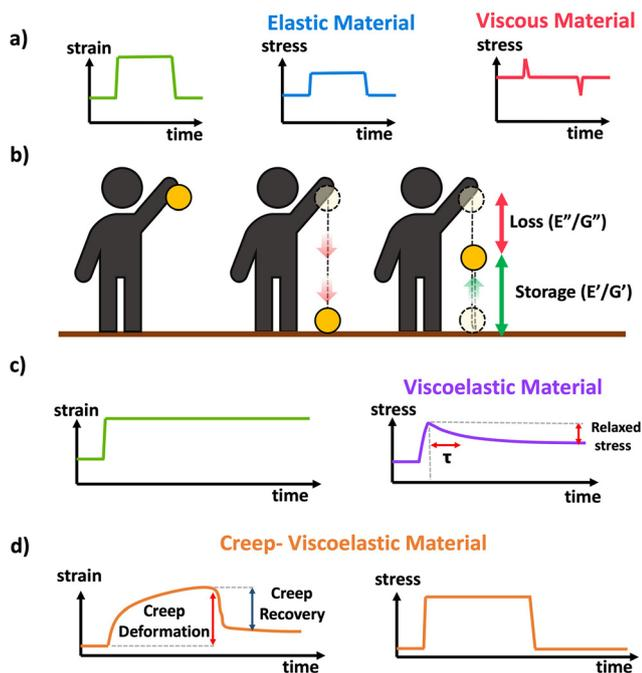
**Scheme 11** (a) Schematic of stress response to strain applied to a perfectly elastic (blue) and perfectly viscous (red) material, (b) conceptual demonstration of viscoelasticity in the context of a ball dropped (image inspired by slide 15 from ref. 89), (c) schematic response of a viscoelastic material to applied strain in a stress relaxation experiment. (d) Schematic response of a viscoelastic material to a transiently applied stress in a creep experiment.
