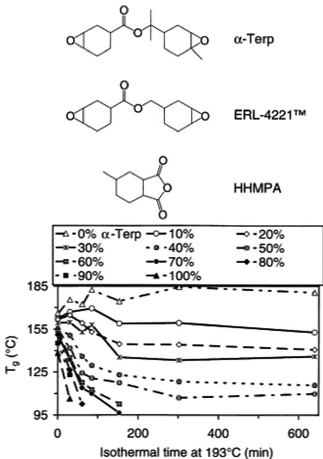
Fig. 7 Glass transition temperatures of the samples used in swelling tests as a function of their rework times. The greater the amount of  $\alpha$ -Terp in the material, the lower the  $T_g$  (reproduced from ref. 105 with permission from Elsevier, copyright 2004).
