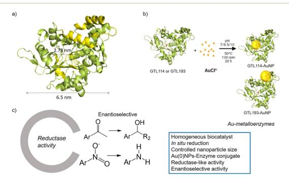
Fig. 1 Schematic illustration of the gold-enzyme conjugate synthesis and reductase catalytic activity. (a) GTL structural dimension, (b) Synthetic approach, (c) Novel reductase-like activity and advantages of the artificial metalloenzymes.
