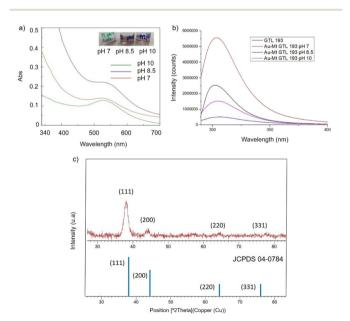
Fig. 4 Characterisation of the different GTI -193 gold metalloenzymes (a) UV-Absorbance spectrophotometer, (b) fluorescence spectra using 280 nm excitation, (c) XRD pattern.
