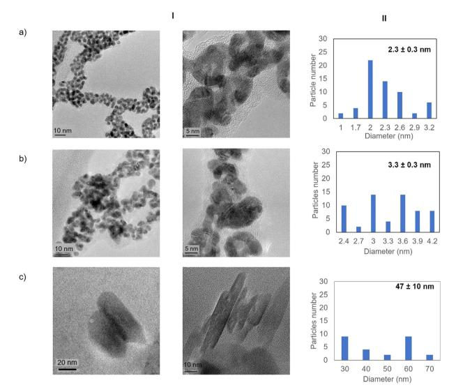
Fig. 3 Electronic microscopy characterisation of the different GTL-114 gold metalloenzymes. (a) Au-Mt@GTL-114 pH 7, (b) Au-Mt@GTL-114 pH 8.5, (c) Au-Mt@GTL-114 pH 10. (l) TEM and HR-TEM, (II) nanoparticle size distribution graphic.
