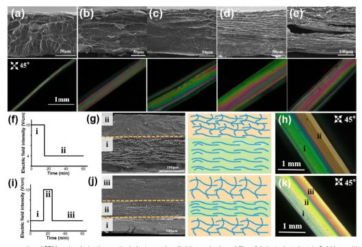
Fig. 3 (a)–(e) Cross-sectional SEM and polarization optical photographs of chitosan hydrogel films fabricated at electric field intensities of 2, 4, 6, 8, and 10 V cm<sup>-1</sup>. The (f) two-step and (i) three-step electrical signal programs used to build E-CS with hierarchical structures. (g) and (j) Cross-sectional SEM images and schematics of the microstructures and (h) and (k) polarization optical photographs of the resultant bi- and tri-layer E-CS, respectively.
