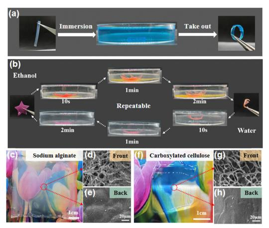
Fig. 5 (a) Qualitative deformation of bilayer E-CS in the  $CuSO_4$  solution and (b) deformation and recovery of pentagram-shaped hydrogels in ethanol and water solutions, respectively. (c) Optical image of the sodium alginate hydrogel and SEM images of its (d) front and (e) back surfaces. (f) Optical image of the carboxylated cellulose nanofiber hydrogel and SEM images of its (g) front and (h) back surfaces.
