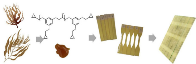
Scheme 1 Chemical formula of PHTE and the so-formed resin and glass fibre reinforced composite images.
