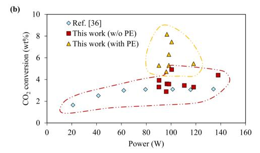
Fig. 5 Effect of PE on  $CO_2$  conversion. (a) Cumulative  $CO_2$  conversion after complete PE conversion under various reaction conditions, and (b) comparison of  $CO_2$  conversion from this work with ref. 36 values.
