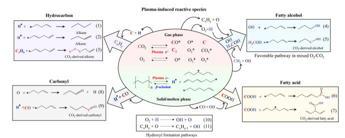
Fig. 6 Proposed reaction pathways of plasma-based co-upcycling of polyolefin and CO<sub>2</sub> with CO<sub>2</sub> or CO<sub>2</sub>/O<sub>2</sub> plasma.
