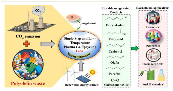
Scheme 1 Concept of plasma co-upcycling waste plastics and CO<sub>2</sub>. CO<sub>2</sub> serves as an oxidant and carbon source to depolymerize polyolefins into platform chemicals, whereas plastics enhance CO<sub>2</sub> conversion. Fatty alcohols are selectively produced by adding O<sub>2</sub>
