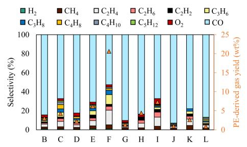
Fig. 2 Gas product selectivity and PE-derived gas yield  $(H_2 \text{ and } C_x H_v)$  for different reaction conditions.
