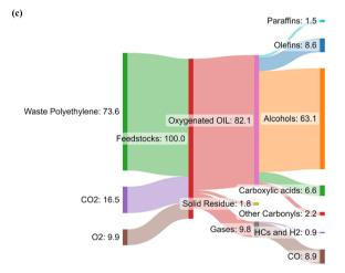
Fig. 7 Plasma-based upcycling of common polyolefins and post-consumer mixed PE. (a) Liquid product composition from conversion of PE, LDPE, PP and PC-PE by (i)  $CO_2$  and (ii)  $CO_2/O_2$  plasma, (b) overall mass balance from PC-PE conversion by  $CO_2$  plasma, and (c) overall mass balance from PC-PE conversion by  $CO_2/O_2$  plasma.
