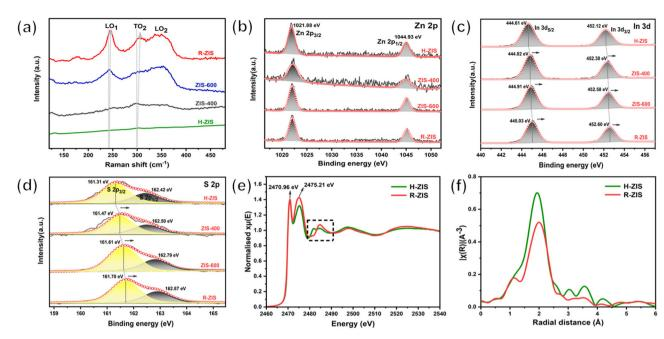
Fig. 3 (a) Raman spectra of H-ZIS, ZIS-400, ZIS-600, and R-ZIS electrodes. (b–d) XPS spectra of Zn 2p, In 3d, and S 2p for H-ZIS, ZIS-400, ZIS-600, and R-ZIS electrodes. (e) Normalised S K-edge XANES spectra and (f) Fourier transform of In K-edge EXAFS spectra in the *R*-space of the H-ZIS and R-ZIS electrodes.
