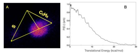
Fig. 7 (A) Sliced velocity map image of the 85 u product,  $C_4H_5S$ , for the reaction of  $S(^3P)$  with isoprene (Newton diagram superimposed) under a collision energy of 11.7 kcal mol $^{-1}$ . (B) Total translational energy release ( $P(E_T)$ ) extracted from image (A).
