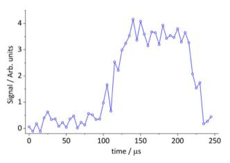
Fig. 5 Time-dependent integrated line intensity of the thioketene  $7_{0,7}$ – $6_{0,6}$  transition at 78.424 GHz, from the reaction of  $S(^3P) + 1,3$ -BD  $\rightarrow$  thioketene ( $C_2H_2S$ ) + ethene ( $C_2H_4$ ).
