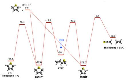
Fig. 2 Stationary points on the PES of the reaction of  $S(^3P)$  with 13BD. Energies in kcal  $mol^{-1}$  are relative to the  $S(^3P)$  +13BD entrance channel at the CCSD(T)-F12a/cc-pVTZ-F12/ $\omega$ B97X-D/6-311++G(d,p) level and include ZPE.
