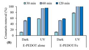
Fig. 9 (A) Effect of FeCl<sub>3</sub> in the presence and absence of E-PEDOT under irradiation (experimental conditions: [hexazinone]<sub>0</sub> = 5  $\mu$ M, [Fe(|||)]<sub>0</sub> = 0.005 and 0.015 mM, pH  $\sim$ 6.5, irradiation time = 60 min, UVC intensity = 20 mW cm<sup>-2</sup>); (B) coumarin removal in the dark and under irradiation in the presence of E-PEDOT and 0.05 mM FeCl<sub>3</sub>.
