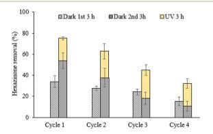
Fig. 7 The reusability of E-PEDOT for hexazinone removal in the dark and under UV irradiation (experimental conditions:  $[hexazinone]_0 = 5$  $\mu$ M, pH  $\sim$ 6.5, UVC intensity = 20 mW cm<sup>-2</sup>).
