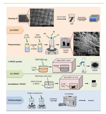
Scheme 1 The polymerisation of E-PEDOT and C-PEDOT for photocatalysis experiments.
