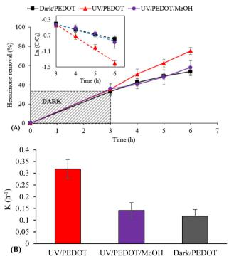
Fig. 6 (A) Hexazinone removal (%) and kinetics in the presence of MeOH; (B) effect of MeOH on photodegradation rate of hexazinone (experimental conditions:  $[hexazinone]_0 = 5 \mu M$ ,  $[MeOH]_0 = 0.5 mM$ , pH  $\sim$ 6.5, UVC intensity = 20 mW cm<sup>-2</sup>).
