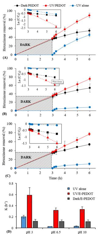
Fig. 5 Hexazinone removal (%) and kinetics at different pHs; (A) pH = 3, (B) pH  $\sim$ 6.5, (C) pH = 10, and (D) hexazinone degradation rate constants at different pHs (experimental conditions:  $[hexazinone]_0 = 5$  $\mu$ M, UVC intensity = 20 mW cm<sup>-2</sup>).
