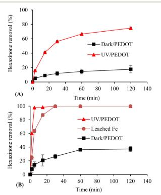
Fig. 8 Hexazinone removal (%) in the presence of (A) immobilised C-PEDOT and (B) C-PEDOT powder (experimental conditions: [hexazinone]<sub>0</sub> = 5  $\mu$ M, C-PEDOT powder dosage = 0.5 g L<sup>-1</sup> pH  $\sim$ 6.5, UVC intensity =  $20 \text{ mW cm}^{-2}$ ).
