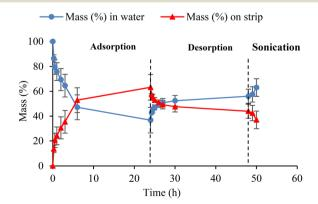
Fig. 4 Adsorption and desorption of hexazinone on E-PEDOT (experimental conditions: [hexazinone] $_0$  = 5  $\mu$ M, pH  $\sim$ 6.5); data are presented as the average of mass (%) adsorbed or desorbed ± standard deviation (N = 2).
