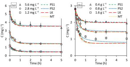
Fig. 4 Effect of initial PO<sub>4</sub>-P concentration on adsorption kinetics for a M@GO dosage of 0.8 g  $L^{-1}$  (a). Effect of M@GO dosage on adsorption kinetics for an initial concentration of 2.8 mg  $L^{-1}$  PO<sub>4</sub>-P (b). Experimental and model results.
