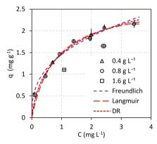
Fig. 3 Adsorption isotherm of PO<sub>4</sub>-P on M@GO at different M@GO dosages.
