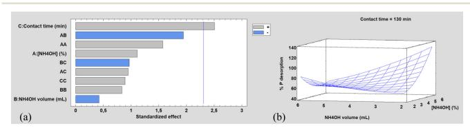
Fig. 6 CCD results: (a) standardized Pareto chart. (b) Response surface. The P desorption percentage is referred to phosphate species.
