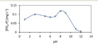
Fig. 1 Effect of pH on aqueous PO<sub>4</sub>-P concentration for a M@GO dosage of 0.8 g L<sup>-1</sup>. The error bars represent 2 times the standard deviation of the aqueous concentrations of triplicate experiments.
