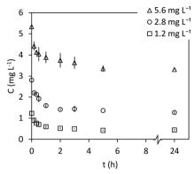
Fig. 2 Effect of contact time on aqueous PO<sub>4</sub>-P concentration for a M@GO dosage of 0.8 g L<sup>-1</sup> and at three different initial PO<sub>4</sub>-P concentrations.
