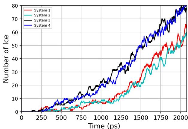
Fig. 6 Time-evolution of the number of ice-like molecules across four parallel simulations (system 1–4).
