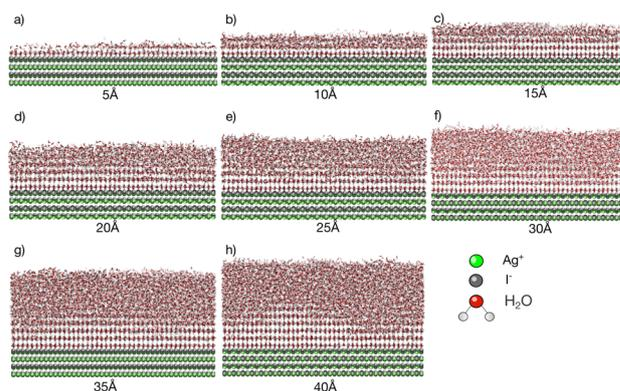
Fig. 1 Snapshots of atomistic MD simulations of TIP4P/Ice water on AgI surface at  $T = 253$  K and  $t = 60$  ns. The thickness of the water slabs is (a) 5, (b) 10, (c) 15, (d) 20, (e) 25, (f) 30, (g) 35 and (h) 40 Å.  $\text{Ag}^+$  and  $\text{I}^-$  ions are colored in silver and green, respectively. TIP4P/Ice molecules are shown as red and white sticks and hydrogen bonds are shown as dashed red lines.
