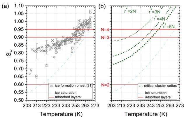
Fig. 7 (a) Compilation of experimentally determined onset conditions ( $S_w$ : water saturation ratio, temperature) for ice nucleation on AgI.<sup>32</sup> (b) Stability conditions for critical ice embryos in water with a radius equivalent to  $N = 2, 3, 4, 5$  adsorption layers. Ice saturation is shown as a dashed line, and saturation conditions for  $N = 2, 3, 4$  layers of adsorption<sup>37</sup> are indicated as solid lines.
