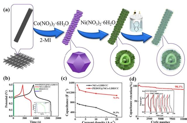
**Fig. 6** (a) Schematic illustration of the preparation of PEDOT@NiCo-LDH/CC. (b) GCD curves of the samples at 1 A g<sup>-1</sup>. (c) Corresponding capacitance at different current densities. (d) Cycling properties of PEDOT@NiCo-LDH/CC at 20 A g<sup>-1</sup> over 10 000 cycles (inset: GCD curves of the first and last 5 cycles). Reprinted with permission from ref. 62, Copyright 2023, Elsevier.
