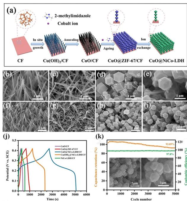
**Fig. 8** (a) Schematic showing the construction of CuO@NiCo-LDH/CF. SEM images of (b and f) Cu(OH)<sub>2</sub>, (c and g) CuO, (d and h) CuO@ZIF-67 and (e and i) CuO@NiCo-LDH on CF. (j) GCD curves at different current densities of CuO@NiCo-LDH/CF, and (k) cycling stability and coulombic efficiency of CuO@NiCo-LDH/CF during 5000 cycles (the inset shows the SEM images of CuO@NiCo-LDH/CF before and after cycling). Reprinted with permission from ref. 74, Copyright 2022, WILEY-VCH.
