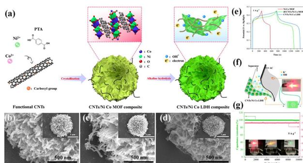
**Fig. 4** (a) Schematic illustration of the synthesis process of the CNT/NiCo-LDH composite. SEM images of the as-synthesized (b) NiCo-MOF, (c) CNTs/NiCo-MOF and (d) CNTs/NiCo-LDH. (e) GCD curves of the as-prepared samples at  $1 \text{ A g}^{-1}$ . (f) Schematic illustration of the CNT/NiCo-LDH//AC hybrid supercapacitor. (g) Cycling performance and the coulombic efficiency of CNTs/NiCo-LDH//AC at  $5 \text{ A g}^{-1}$ . Reprinted with permission from ref. 51, Copyright 2021, Elsevier.
