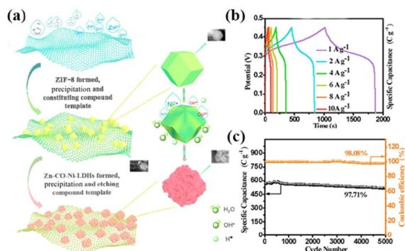
**Fig. 5** (a) Schematic illustration of the synthesis of GO/Zn-Co-Ni LDH. (b) GCD curves of GO/Zn-Co-Ni LDH. (c) Cycling stability and coulombic efficiency of GO/Zn-Co-Ni LDH during 5000 cycles at  $10 \text{ A g}^{-1}$ . Reprinted with permission from ref. 54, Copyright 2020, American Chemical Society.
