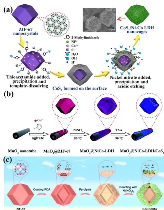
Fig. 7 (a) Schematic illustration depicting the preparation of CoS<sub>x</sub>/Ni-Co LDH composites. Reprinted with permission from ref. 65, Copyright 2019, Elsevier. (b) Schematic diagram outlining the synthesis of MnO<sub>2</sub>@NiCo-LDH/CoS<sub>2</sub>. Reprinted with permission from ref. 66, Copyright 2019, the Royal Society of Chemistry. (c) Schematic illustration demonstrating the synthesis of C/N-CNMA. Reprinted with permission from ref. 70, Copyright 2023, Elsevier.
