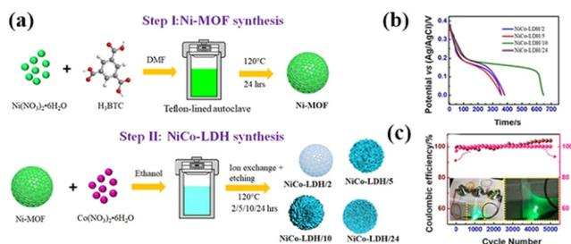
**Fig. 3** (a) Schematic diagram of the synthesis of the Ni-MOF template and derived NiCo-LDHs. (b) GCD curves of NiCo-LDH at 1 A g<sup>-1</sup>. (c) Cycling performance and the coulombic efficiency of NiCo-LDH/10//CNT at 4 A g<sup>-1</sup>. Reprinted with permission from ref. 37, Copyright 2020, American Chemical Society.
