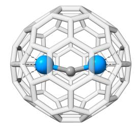
Fig. 9 PBE0-D4/def2-SVP optimized geometry of the U2C@C80-cluster.
