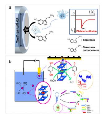
Fig. 3 (a) Schematic of single platelet detection based on the oxidation of the encapsulated serotonin. Reproduced with permission from ref. 91. Copyright American Chemical Society, 2020. (b) Illustration of the detection of the catalytic current of a single GQH during a collision with the Au UME and HCR-based detection of microRNA-15. Reproduced with permission from ref. 94. Copyright American Chemical Society, 2021.
