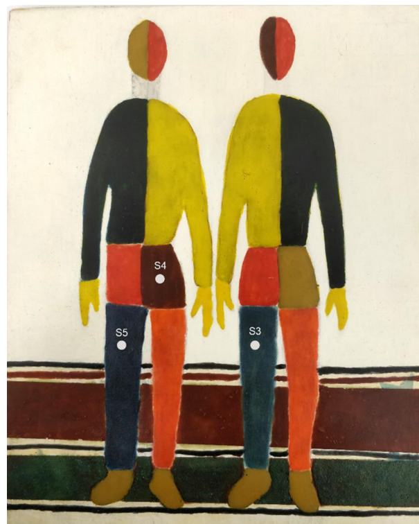
Fig. 1 Laboratory-prepared painting used to demonstrate the potential of portable fibre bundle micro-SORS coupled with serds (see ref. 22 for more details), with indication of the analysed areas (S3–S5).
