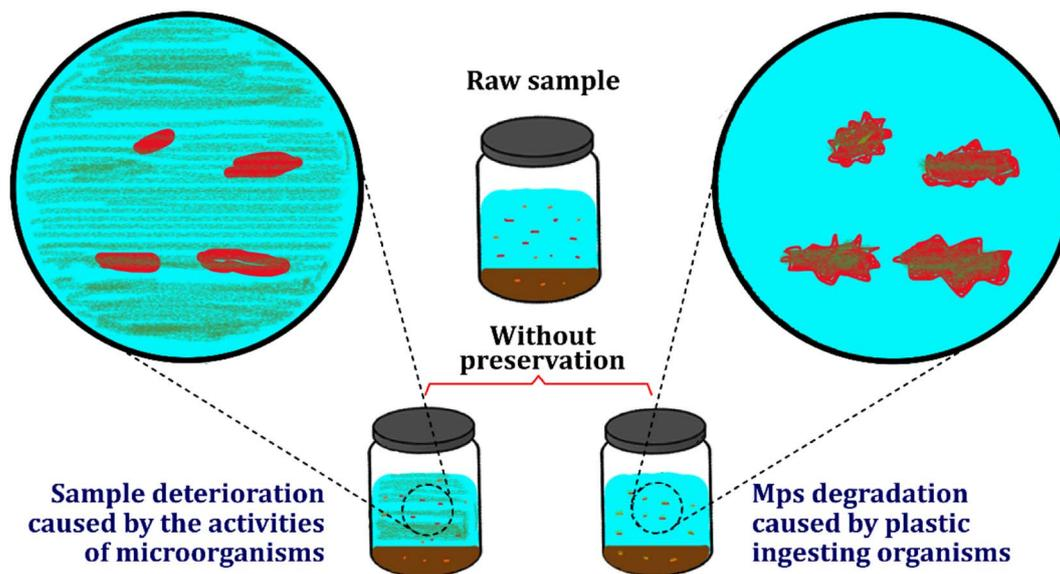
Fig. 5 Schematic of bacterial effect on unpreserved samples.
